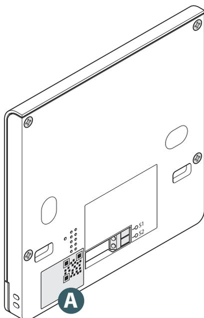
At the rear of the **Unisenza Plus UFH Thermostat RF** there is a sticker **(A)** which indicates the device data.
