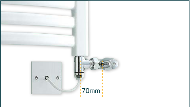
Dual fuel heater kits pipe centre adjustment.
